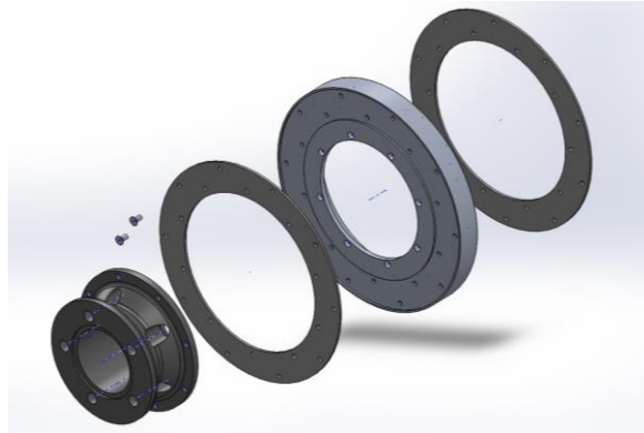
Figure 1: Initial Rotor Design with Off-the-Shelf Rotor/Bearing Carrier
