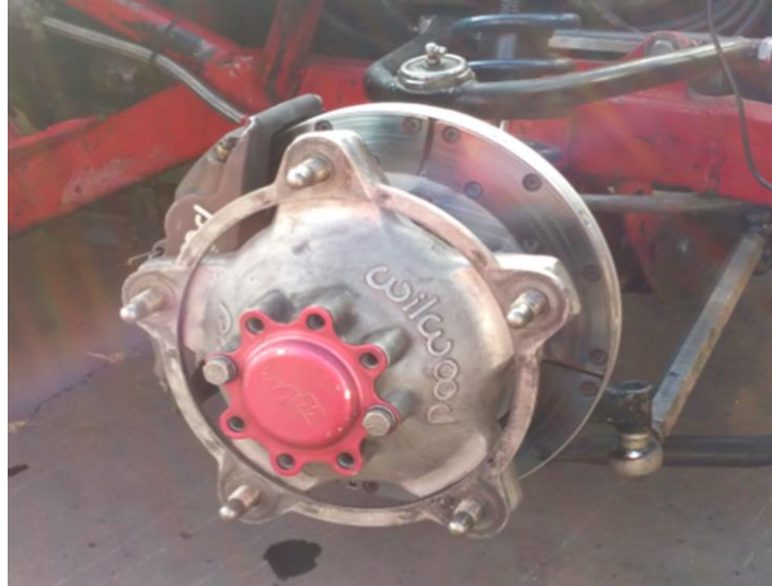
Figure 15: Fabricated Rotor Mounted to Car
