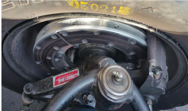
Figure 17: Rotor Condition after 1st Lapping Session
