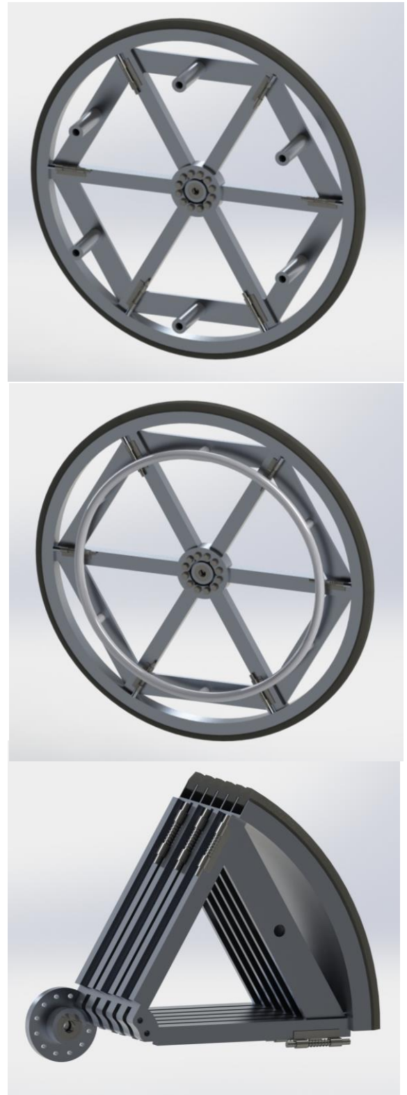
FIGURE 9: 6-piece wheel design 2.0. Attachable handle push rim configuration (Top), attachable circular push rim configuration (Middle), and collapsed configuration (Bottom).
