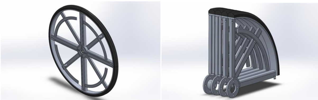
FIGURE 5b: Version 1.1 CAD model of the 4-piece 8-spoke collapsible wheel in an open (left) and closed (right) position.
