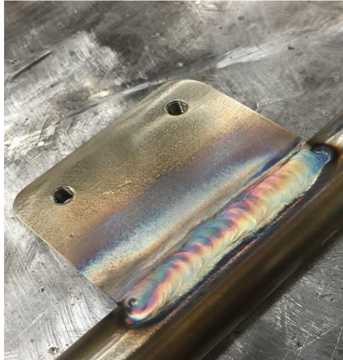
Figure 6: Welded Shaft Assembly
