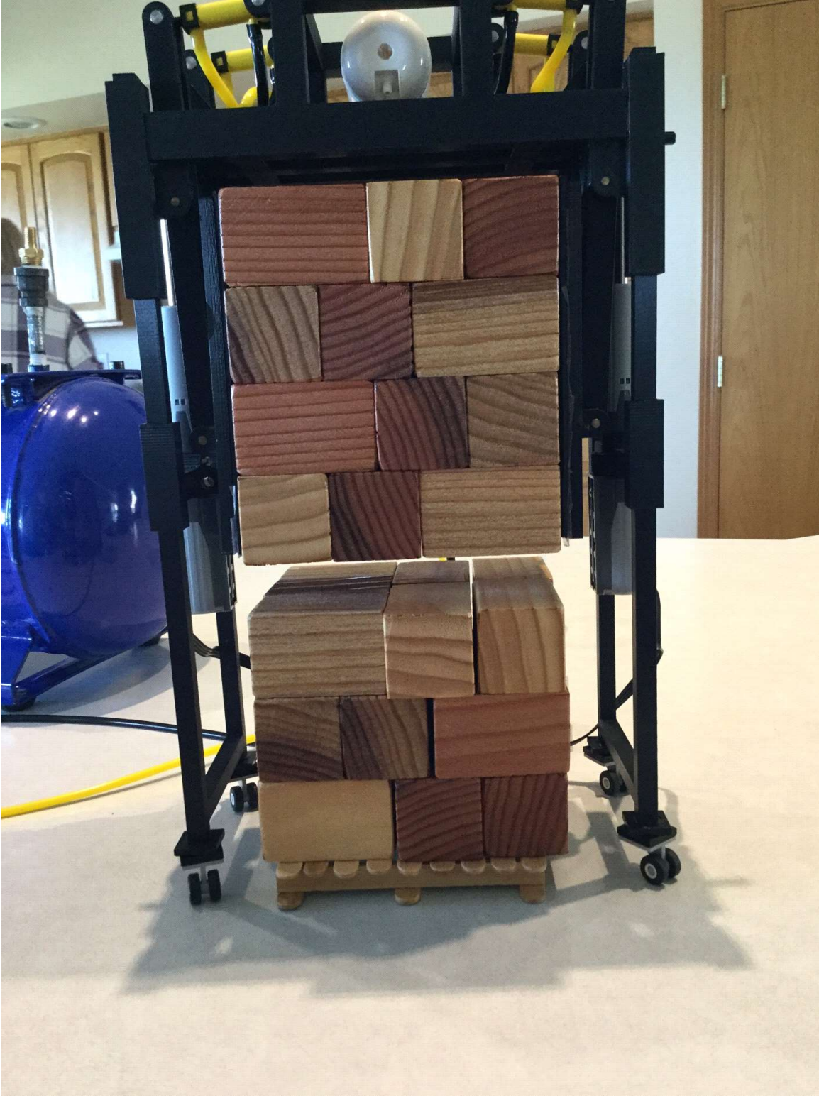
Image 2: This image shows the mini apple boxes lifted at a pressure of 40 psi.
