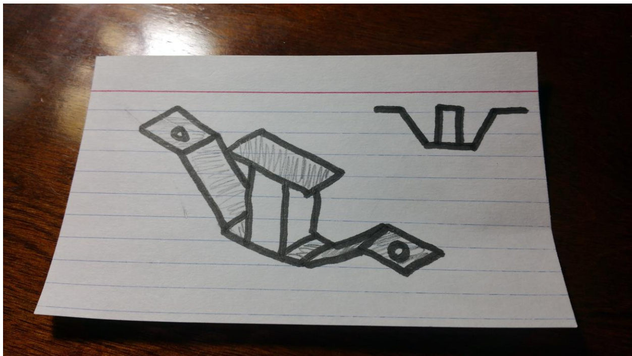
Figure 1: Original design of the attachment on the dyno
