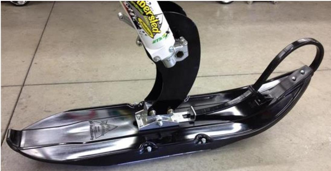
**Figure 4:** Timbersled BackCountry front ski setup for a dirt bike.
