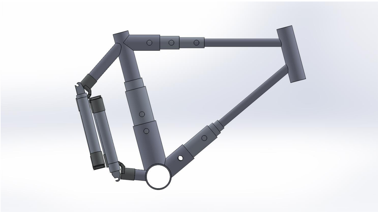
Figure B-1d: Right view of Collapsed Frame
