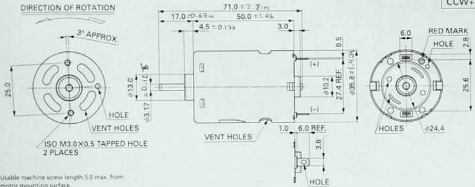
Usable machine screw length 5.0 max. from motor mounting surface.
