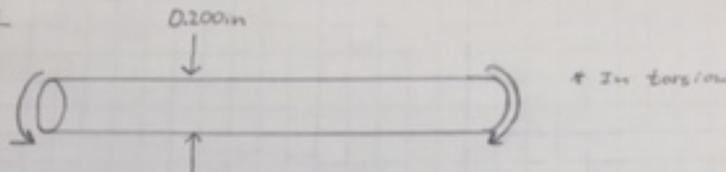
Torque:  $T = \frac{63,000 (0.06 \text{ HP})}{3,500 \text{ rpm}} = 1.08 \text{ in-lb}$
