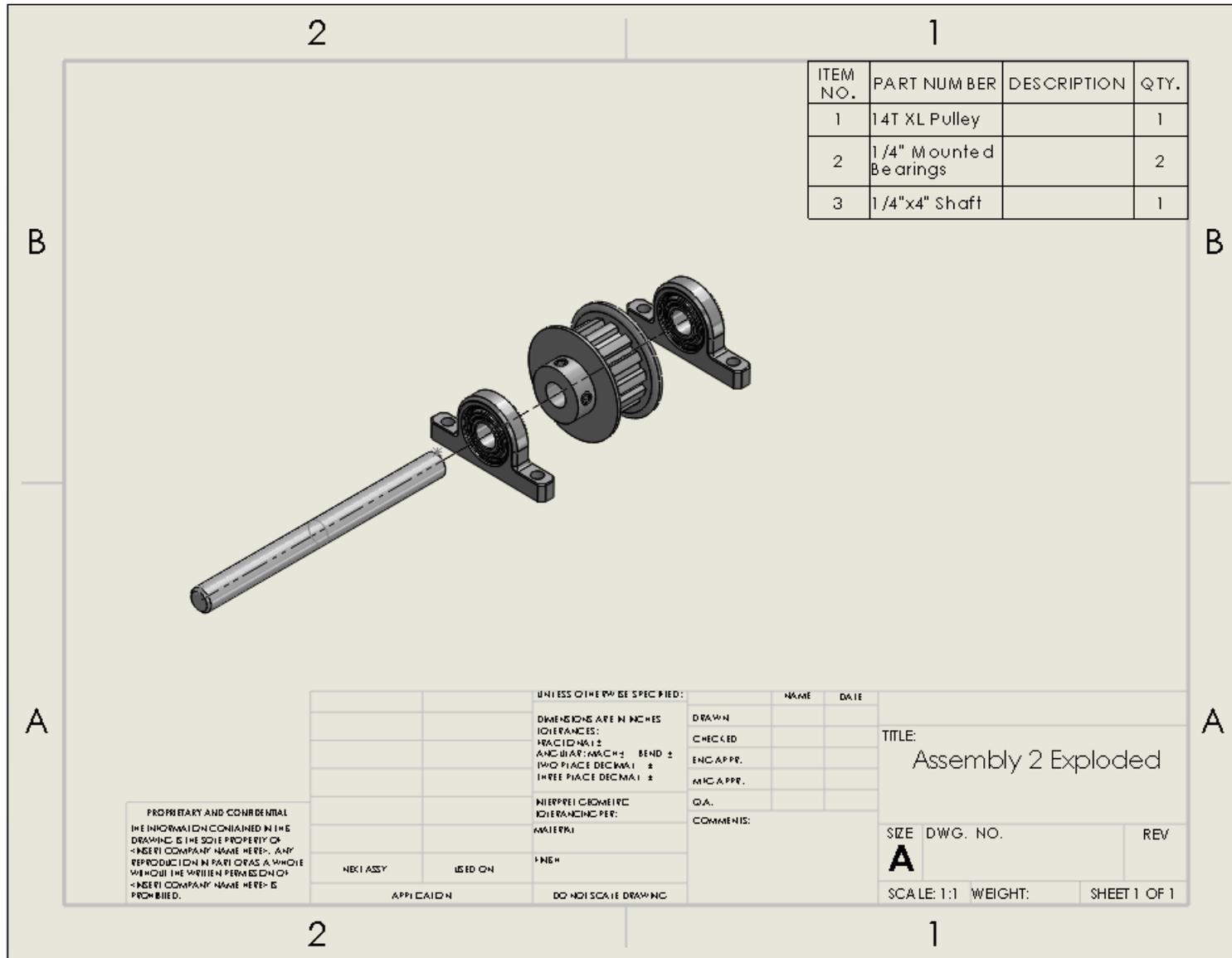
Drawing 10: Timing Pulley Rear Axle
