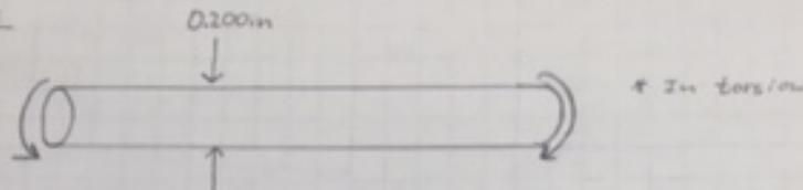
Torque:  $T = \frac{63,000 (0.06 \text{ HP})}{3,500 \text{ rpm}} = 1.08 \text{ in}\cdot\text{lb}$
