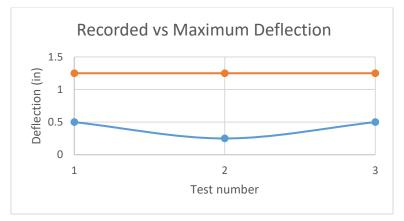
As shown in the graph, the most the back end of the car deflected was 0.5 inches. This means all three tests were successful.
