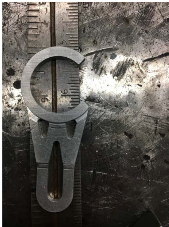
B15 Part after 2 hours in tumbler.
