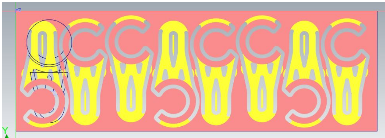
B10 View of 8 parts nested and verified in 4"x12" stock material
