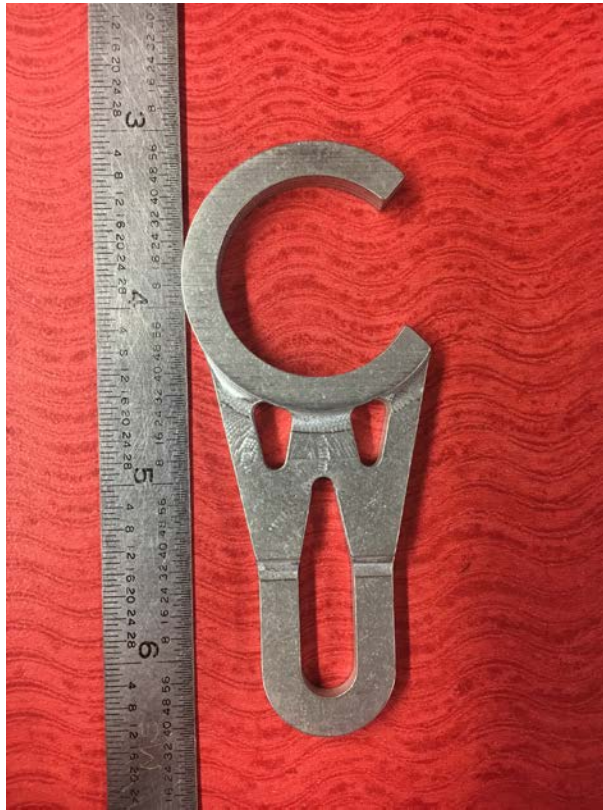
B16 Part after 3 hours in tumbler.
