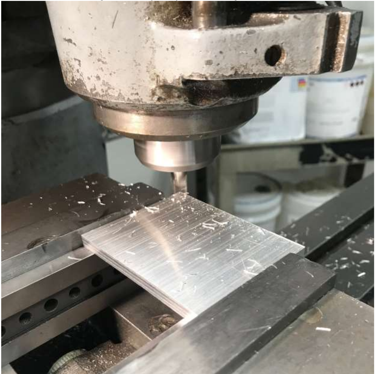
Figure 43 - Photo of the suspension mount being drilled to size
