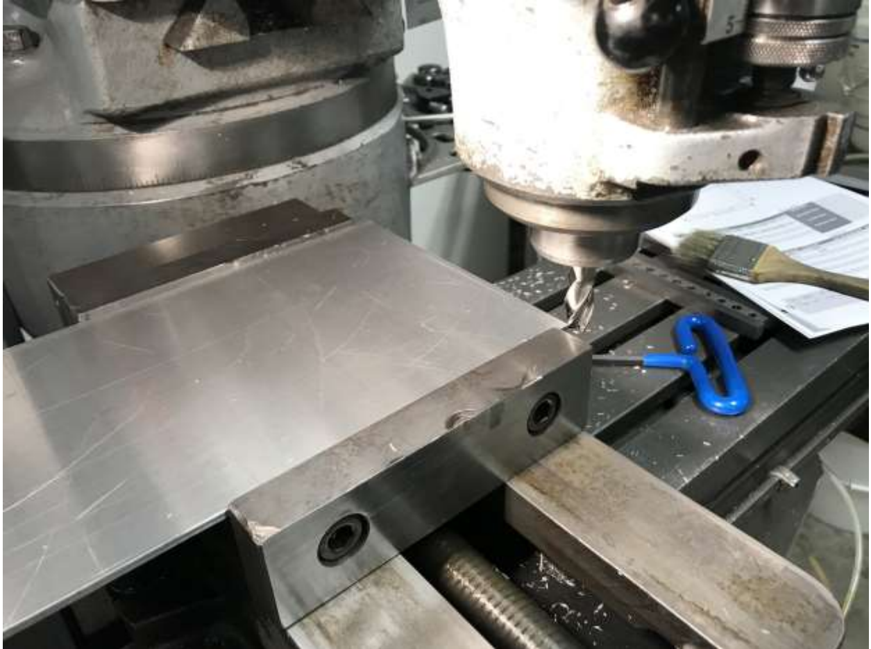
Figure 41 - Photo of the chassis plate being milled to size
