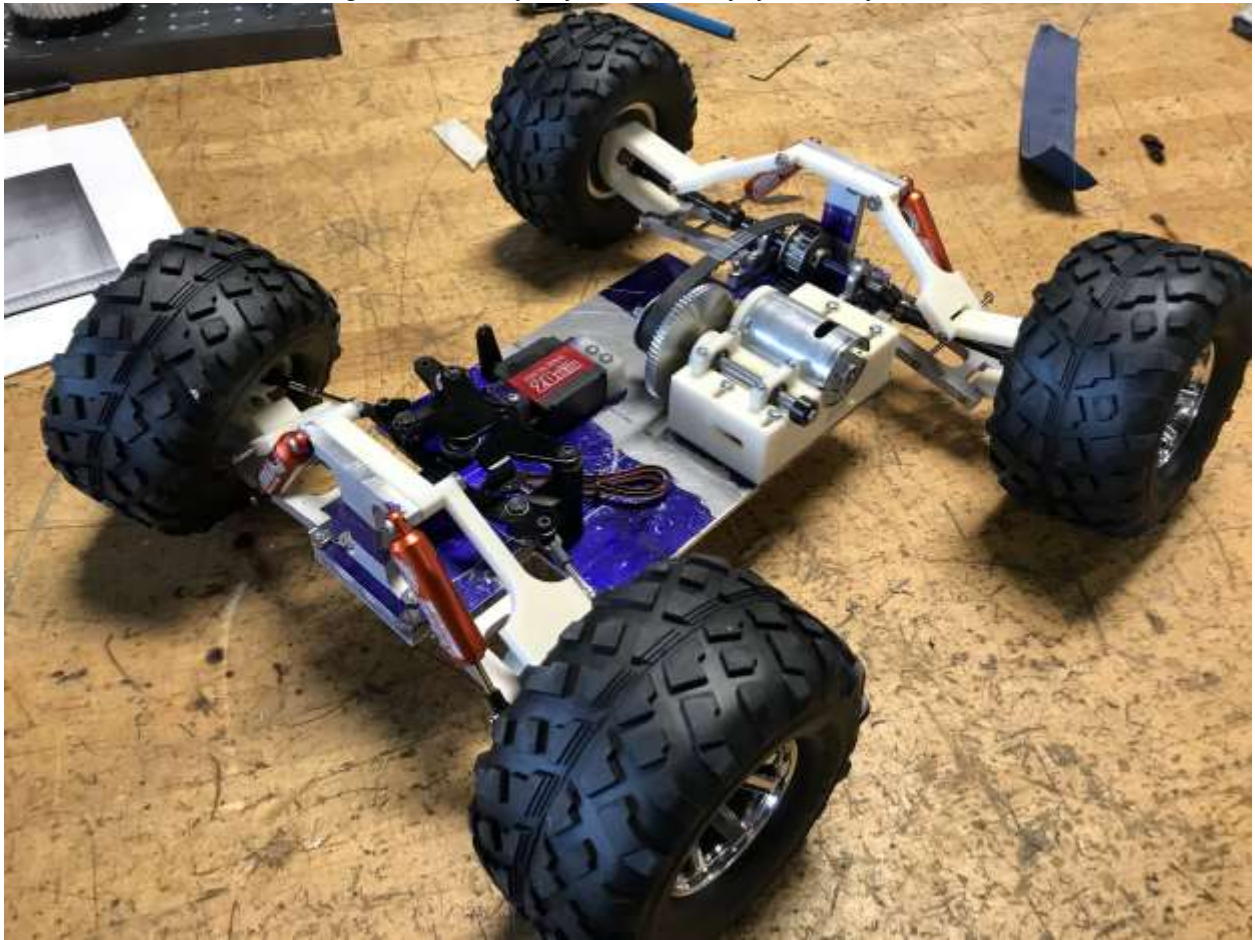
Figure 47 - Photo of the finished assembly of the RC Baja car
