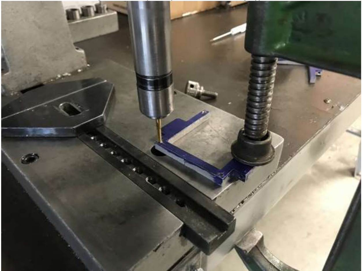
Figure 45 - Photo of the suspension mount holes being tapped
