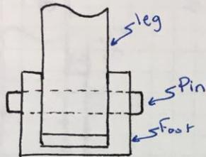
Force of leg onto pin is 3751b
