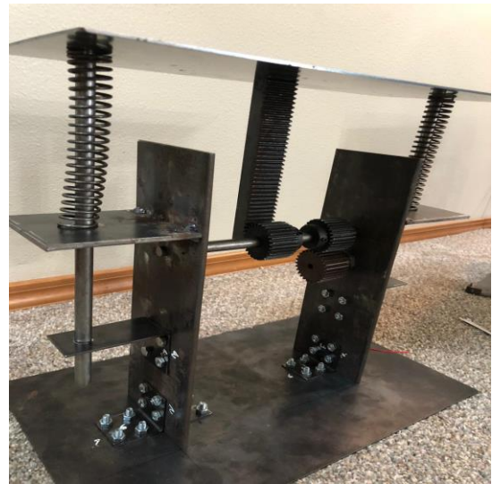
A2) Design (Sketch for rack and pinion with shaft and rod Supports).
