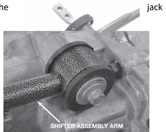
10. From inside the car, carefully pull the shifter assembly out. This is a little bit of a trick so take time, making sure not to scratch or bend center console.
