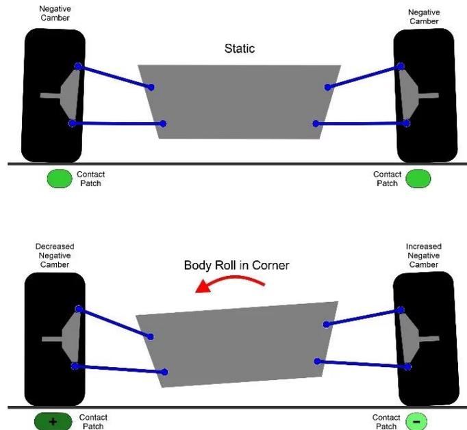
*Figure 2: Contact when cambered*
