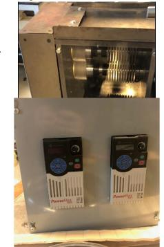
tachometer on lead to a difficulty in obtaining a steady measurement, but the reading leveled out at around 620 rpm. This value was very close to the calculated value of 613 rpm. However, the test was considered a fail because the required rpm for the test to be successful was much lower, at 9.6 rpm.
