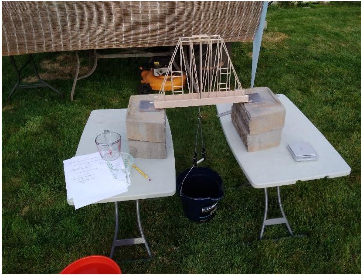
Figure 8: Load Testing Setup
