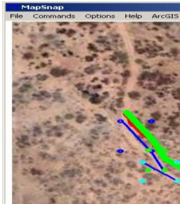
Figure 10. Road extraction using ASA-DLP approach with GMTI guidance
