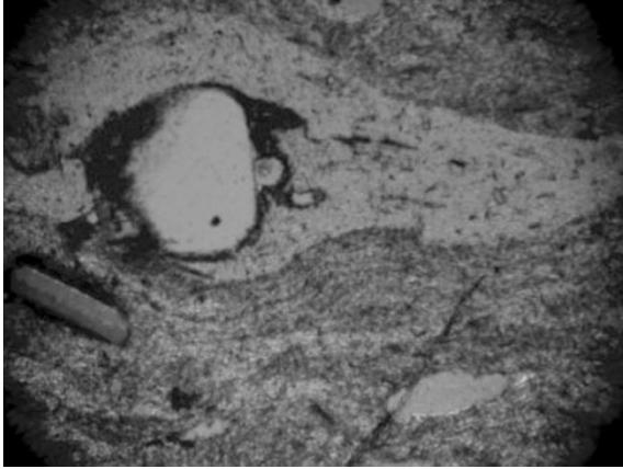
Fig. 15. Photomicrograph demonstrating ignimbritic texture—site sc09: Site sc09 reveals flattened pumice (fiamme) and textural banding, characteristic of an ignimbrite (40X).
