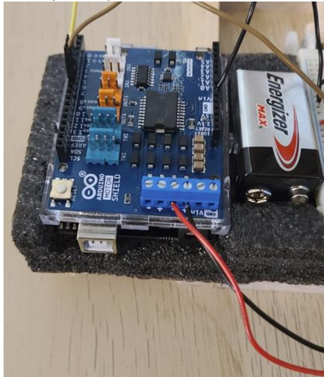
Figure G3 – Motor jumper wires into Arduino
