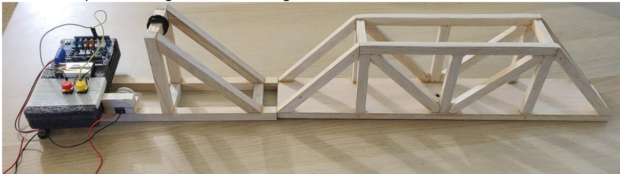
Figure G1 – Articulating Balsa Wood Bridge
