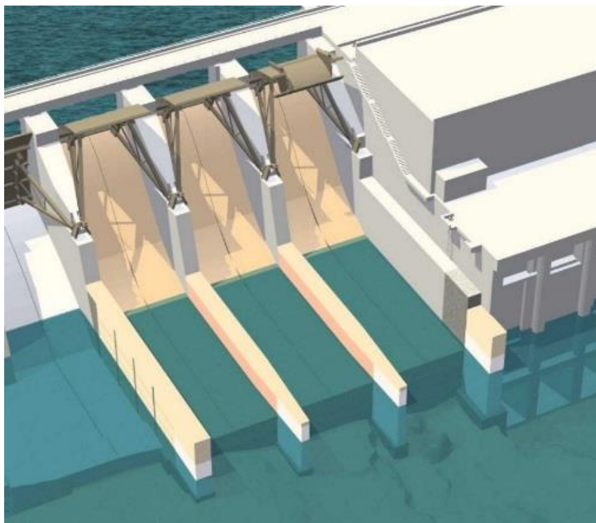
Figure 1: The Priest Rapids Fish Bypass (PRFB). Showing the three surface-spill bays next to the powerhouse.
