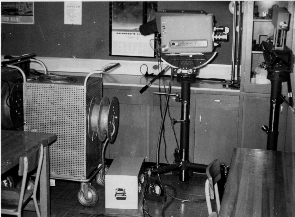
FIGURE 1 TWO CHANNEL CAMERA CHAIN IN A CLASSROOM (FRONT VIEW)
