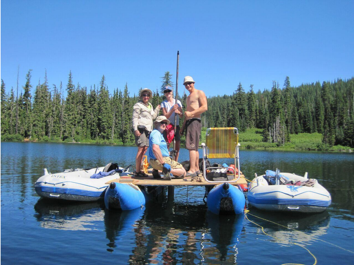
Figure 4.2 Coring from floating platform at Blair Lake, July, 2012.
