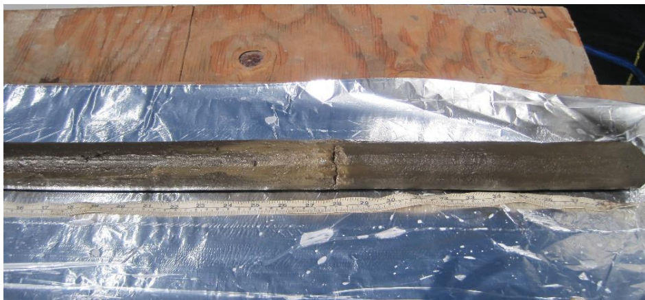
Figure 4.1 Extruded long core drive from Blair Lake.
