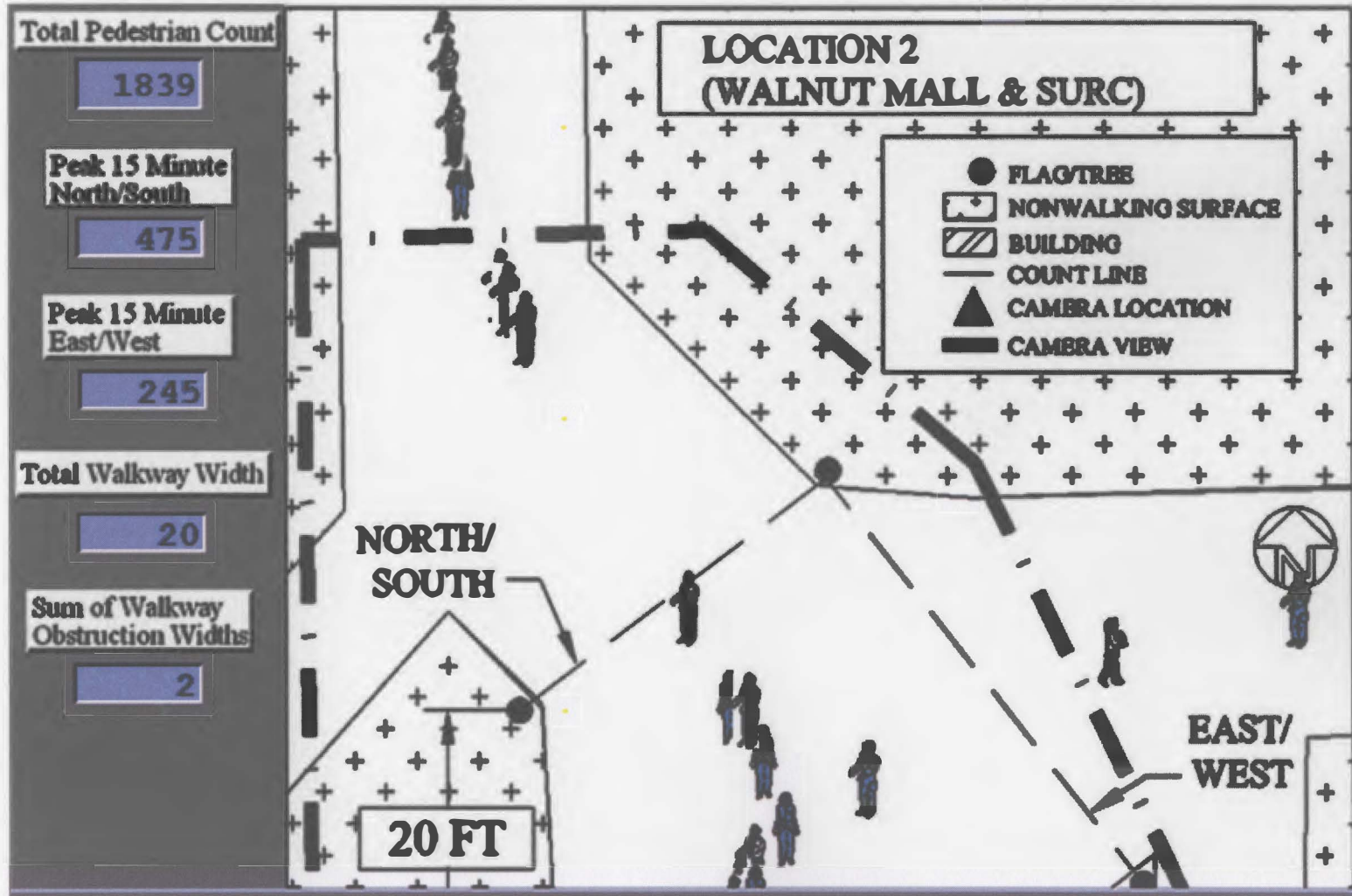
Figure 8. ProModel simulation model screen shot of Location 2 (Student Union and Recreation Center [SURC]).
