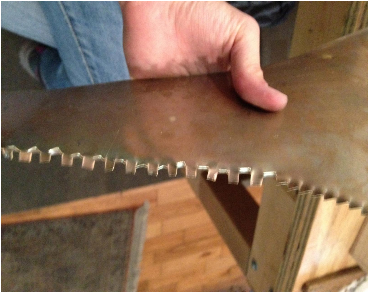
Teeth cut and folded along one side of the bell piece
