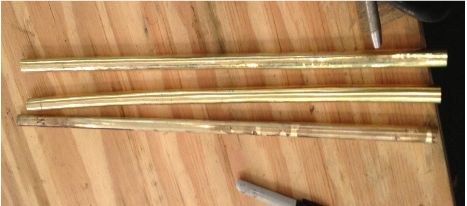
Two polished pipes (top) and one unpolished pipe (below)
