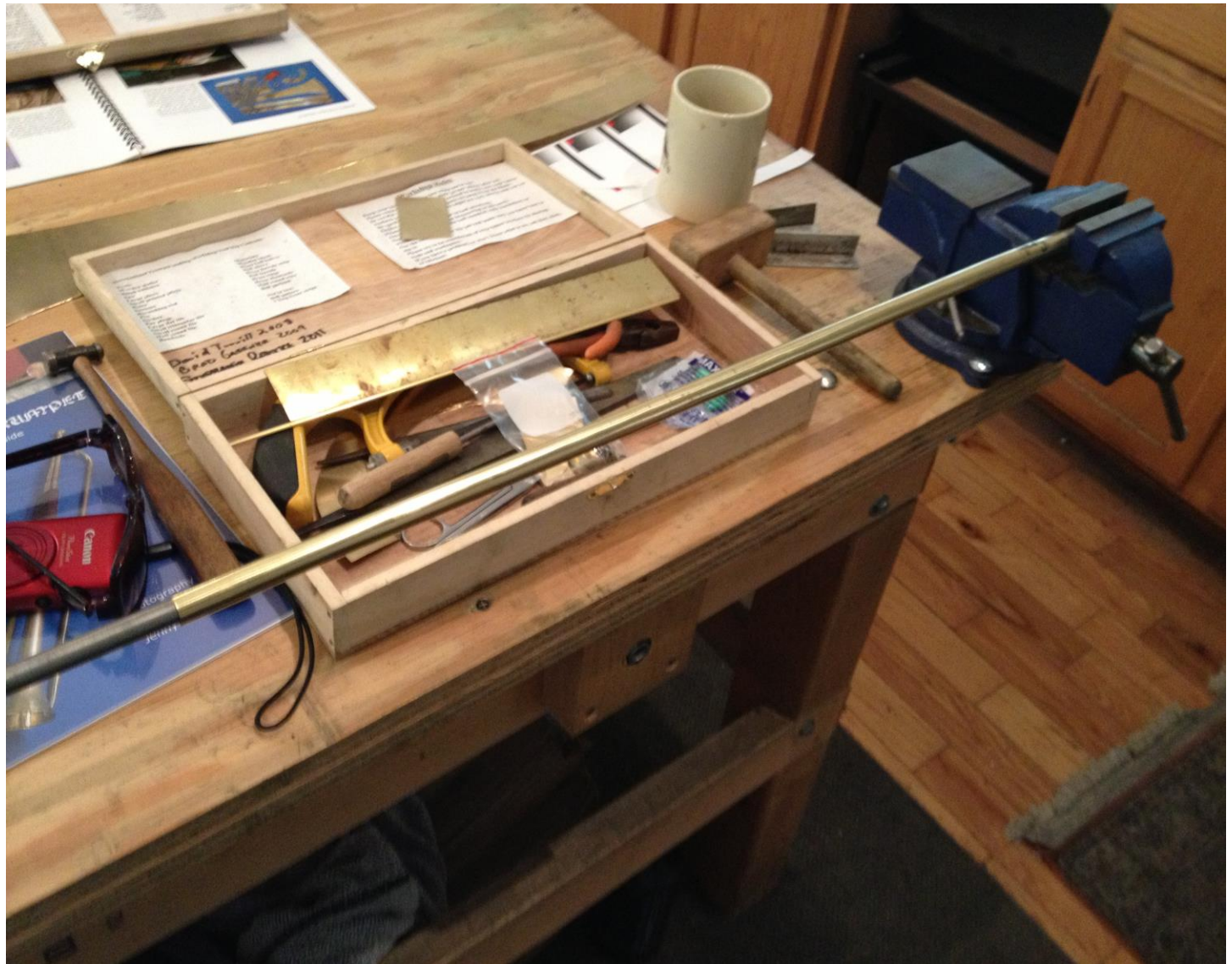
A soldered tube on the mandrel, ready for burnishing and polishing
