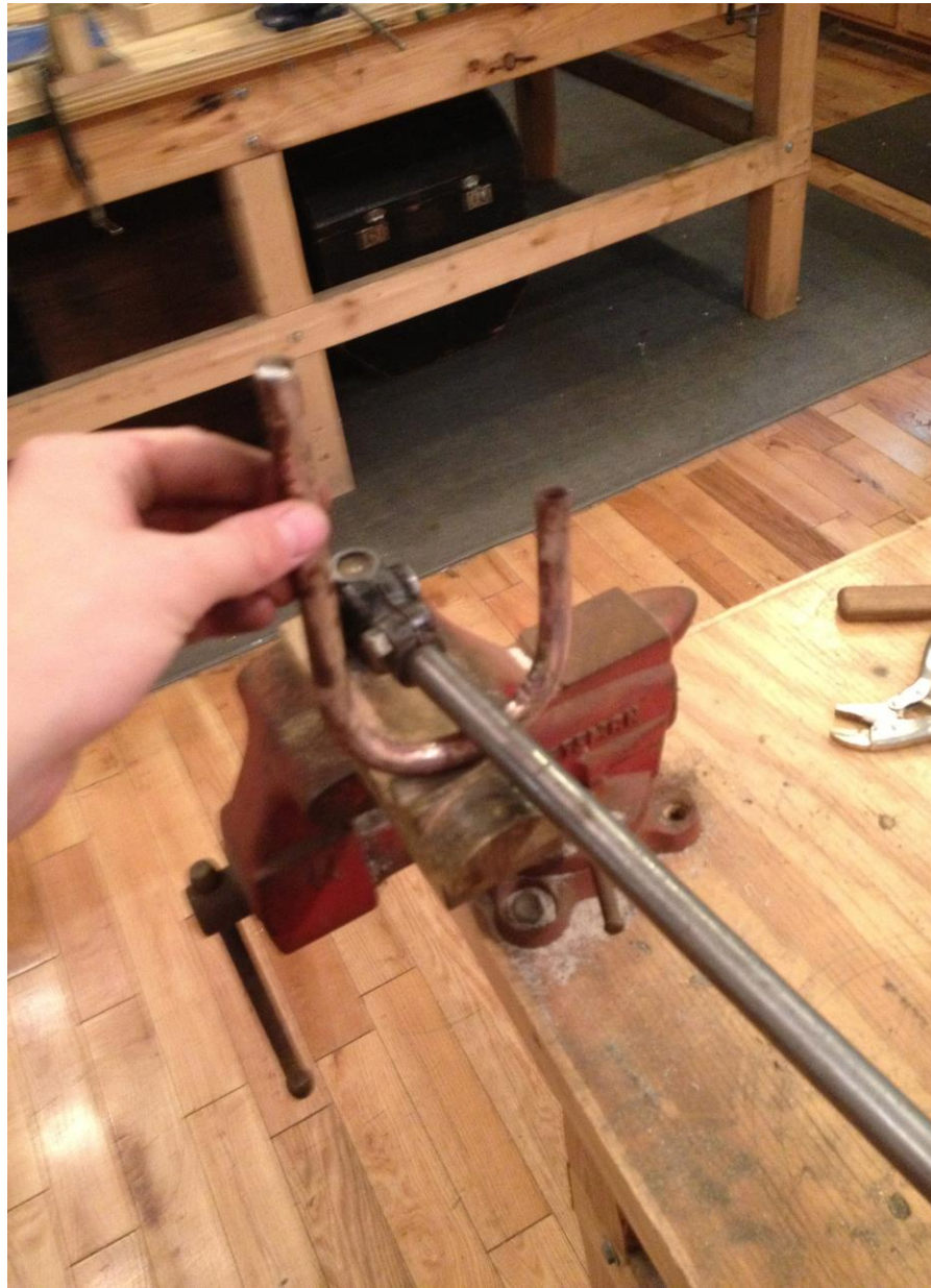
Smoothing out my newly bent bows with a burnishing rod and bench vice
