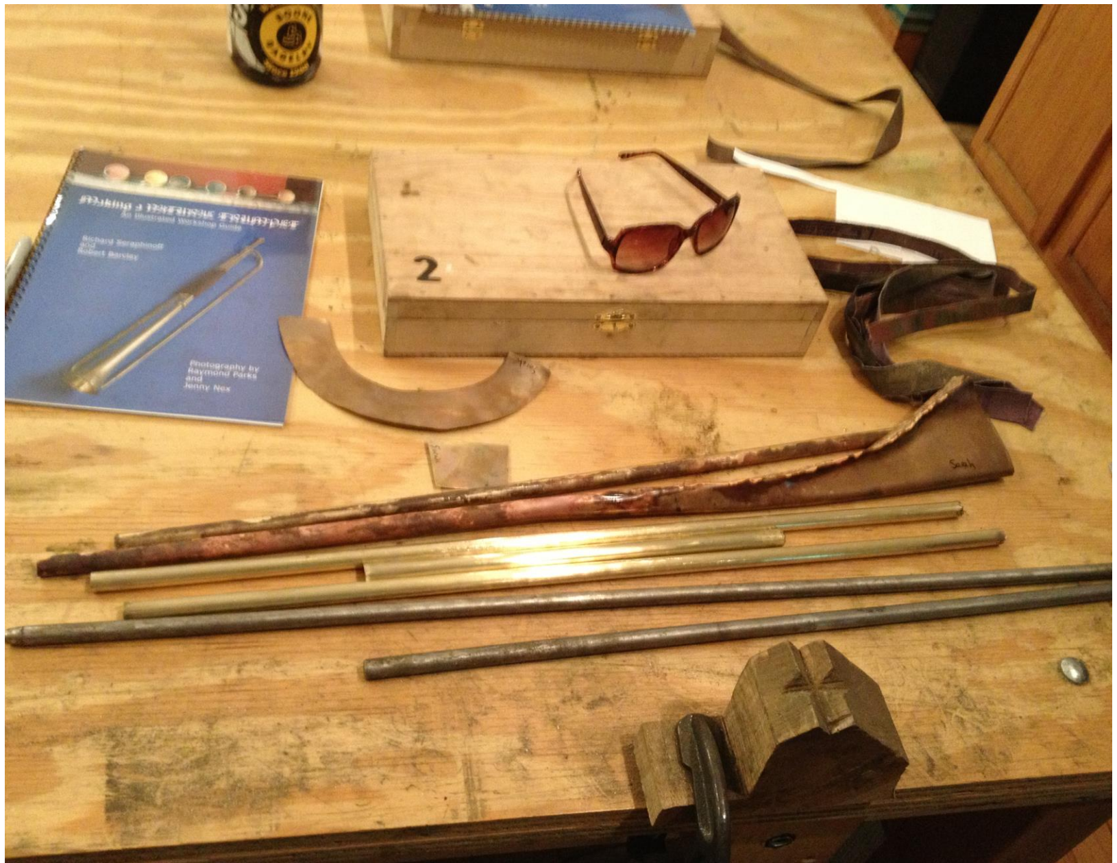
Work completed after day one: three polished pipes, one unpolished pipe, and a folded and soldered bell piece
