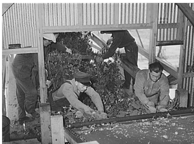
Figure 143. Hop vines going in stationary-type mechanical picker. Putting vines on hooks to begin their journey through the stationary picking machine, where fingers comb hops off the vines. Yakima Chief Hop Ranch. (Russell Lee, 1941), believed to be ~ 1950 or later.
