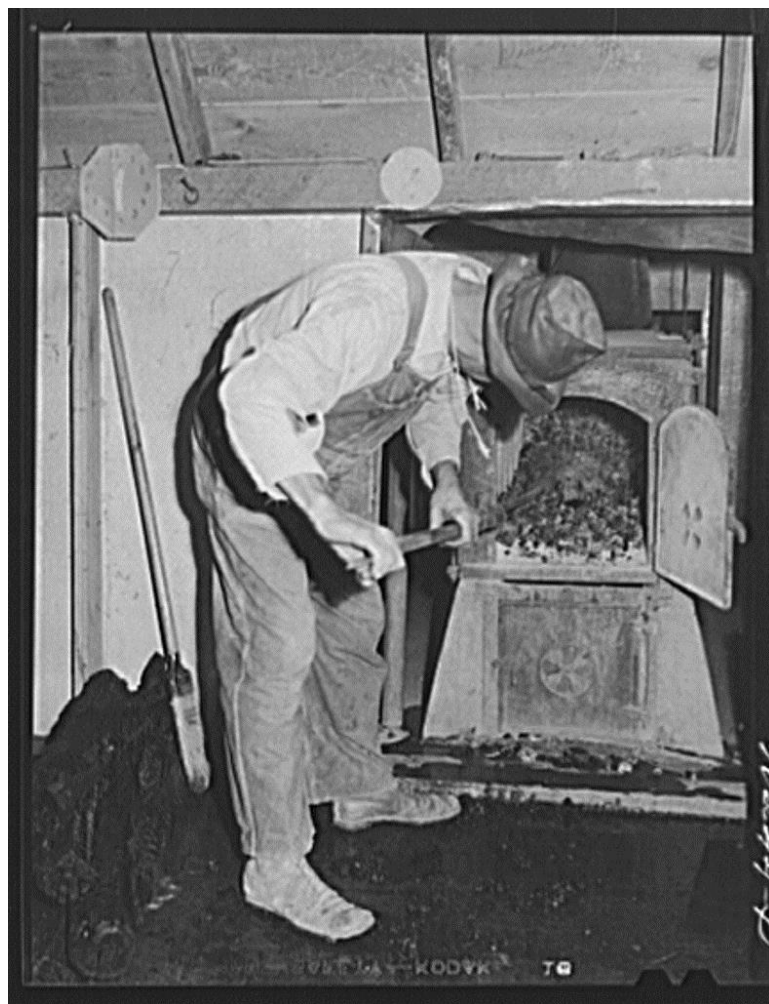
Figure 119. Fixing the fire at the hop kiln. (Russell Lee, 1941, Yakima County). LC-USF34-070244 . Most kilns had several stoves below the kiln. This was one of the most important jobs in the kiln.
