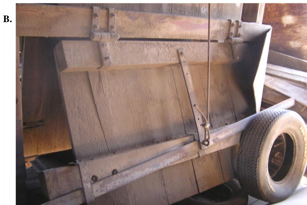
Figures 132. Hop press inside the Paul Patnode Kiln. A. Press shown from the ceiling. B. Press shown from the floor of the baling room. The doors come down to provide the proper size shoot for creating the 200 lb. hop bales. (Terri Towner, 2010)
