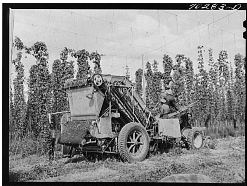
Figure 141. Portable-type mechanical hop picker. Yakima County, Washington. ( Russell Lee, 1941) Yakima Chief Hop Ranch, Tonnenish. WA.
