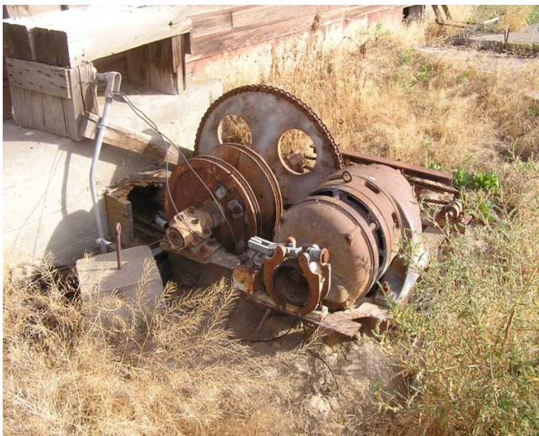
Figure 128. Horse-drawn actuator for the press at the O. J. Gendron Ranch. One or two horses would be hitched to this and would go round and round until the bale was pressed. When given the command the horse(s) would turn and go the opposite direction to pull the press back up to its highest position. The small door on the building leads directly into the press. (Terri Towner, 2016)
