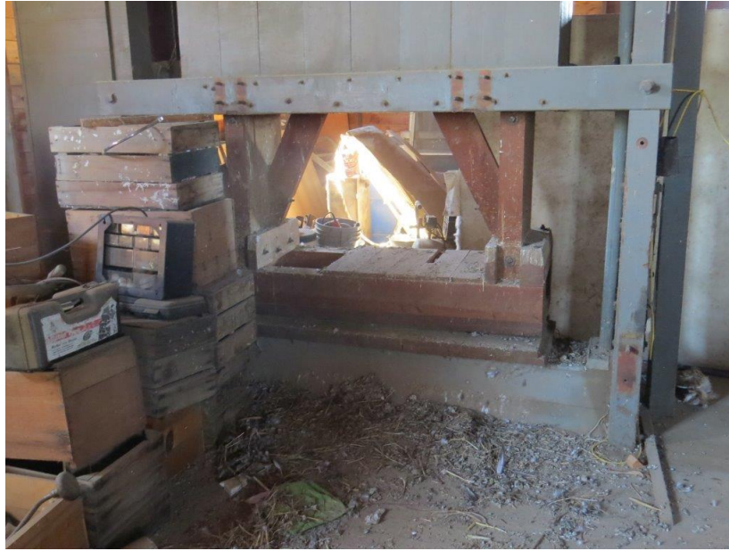
Figure 130. Hop press in the O. J. Gendron baling room. The doors have been removed. The press is normally clean and well-oiled to keep the lupulin from the hops from sticking to it. Burlap was spread on the bottom of the press and then wrapped around the bale and sewn. Helen and Genevieve Duffield took on this job while their husbands worked the press from above. (Terri Towner, 2016)
