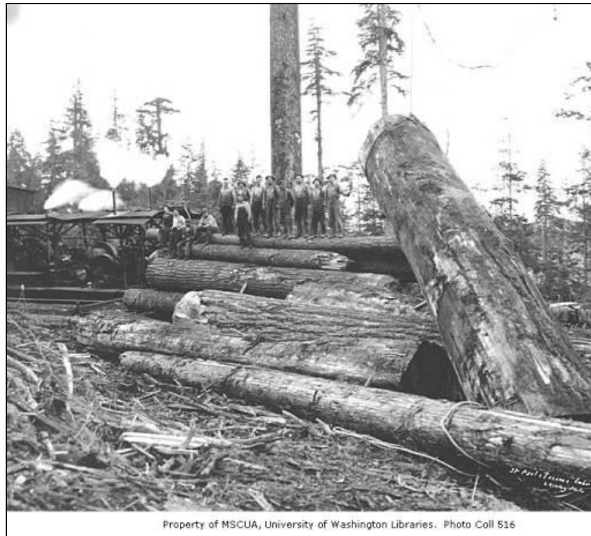
Figure 17. Undated photograph of SPTLC yarding crew and steam donkey engine beside a pile of logs (C. Kinsey 2017d).
