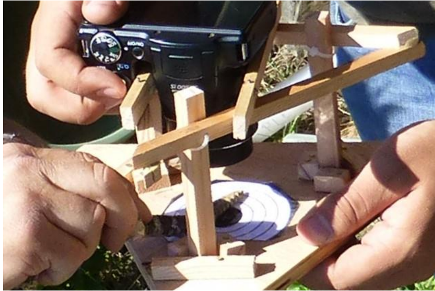
Figure 9: Camera stand setup made to ensure all images were taken at the same distance and angle to allow for accurate measurements, using a black and white target for contrast to maintain the outline of the rattle.
