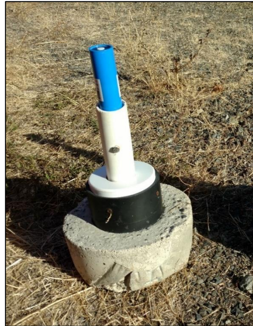
Figure 12. Benthic PAR sensor rig for seafloor readings.
