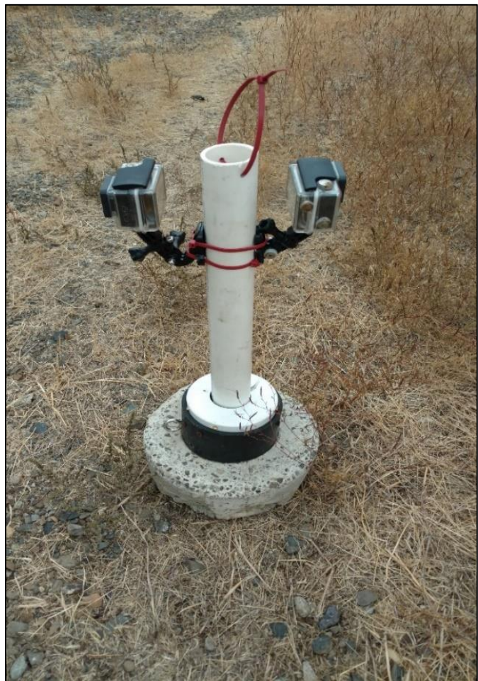
Figure 17. GoPro video set-up for fish use monitoring.
