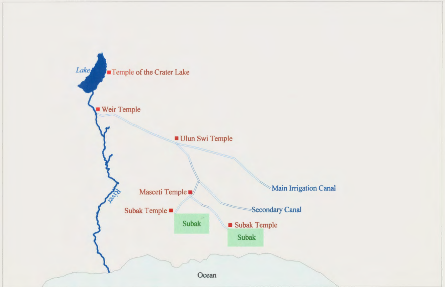
Figure 9: The Balinese rice agricultural irrigation system (Figure is not to scale nor based upon a specific canal system on Bali).
