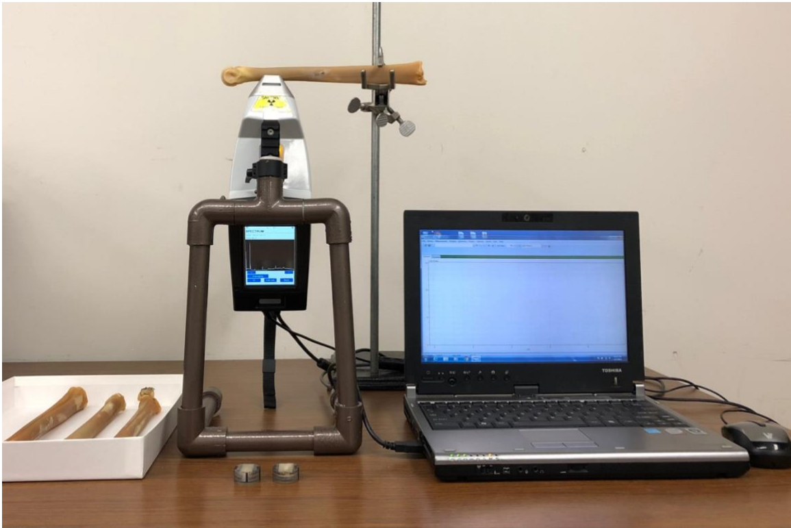
Figure 3.02: Example setup of pXRF, bone specimen, and stands. Photograph by author.
