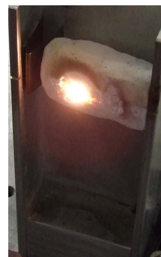
Figure 2. Generating \text{CO}_2 laser radiation as observed on a beam stop.
