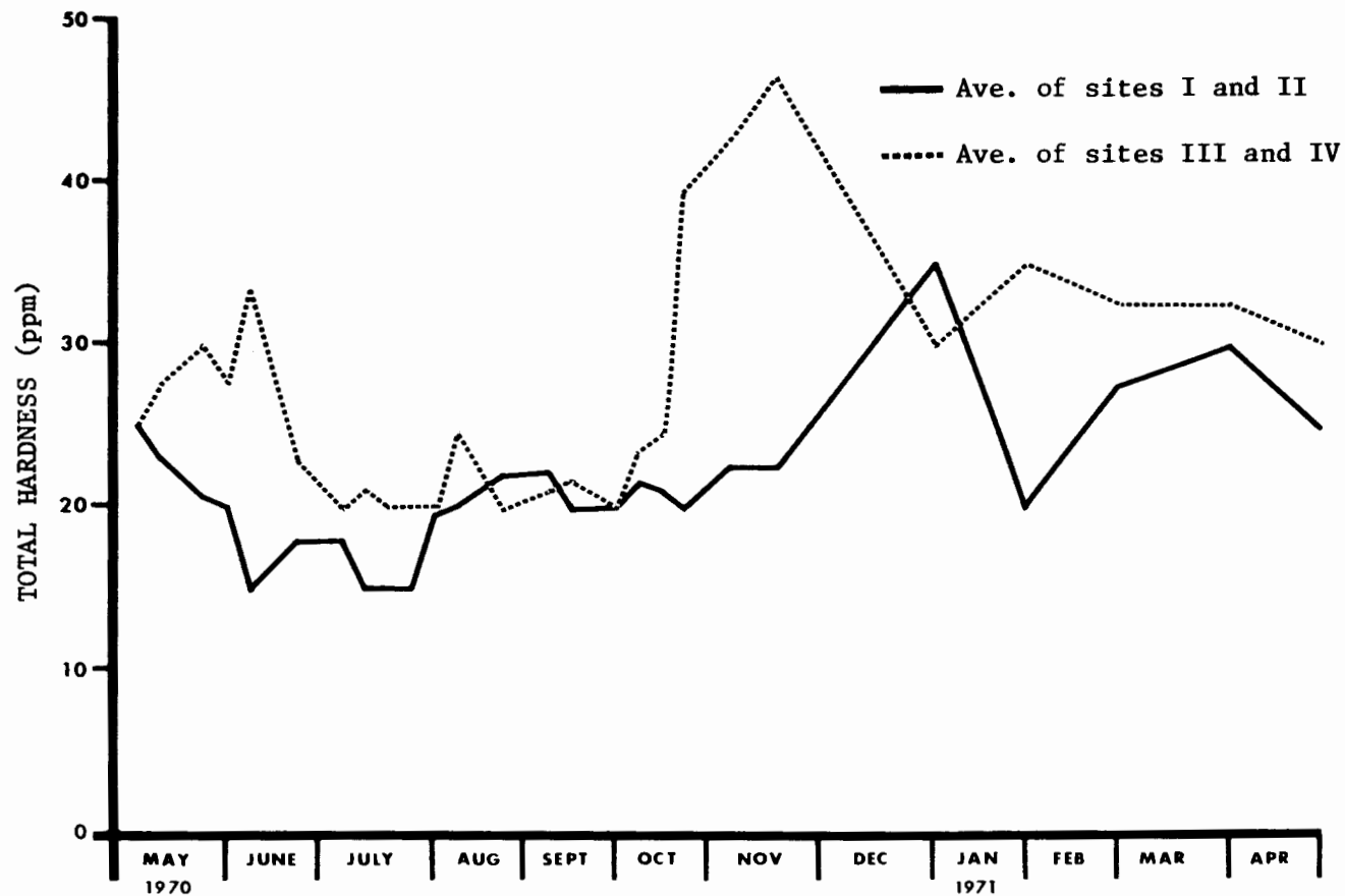
Fig. 11. A comparison of total hardness above and below the reservoir.
