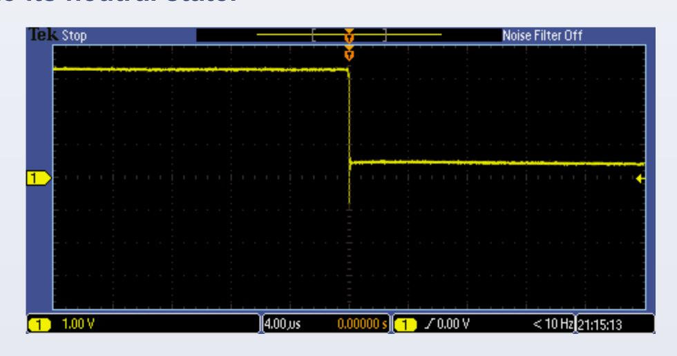
Image 2) This image shows the response time of the Buttons when they are pressed. The signal is held HIGH at 3.3V until the connection is made and circuit goes LOW. The Pi in turn registers that specified response as a specific key press. The signal will be held LOW for about 12µ seconds. It will then return to 3.3V regardless of if the button is continually held down.
