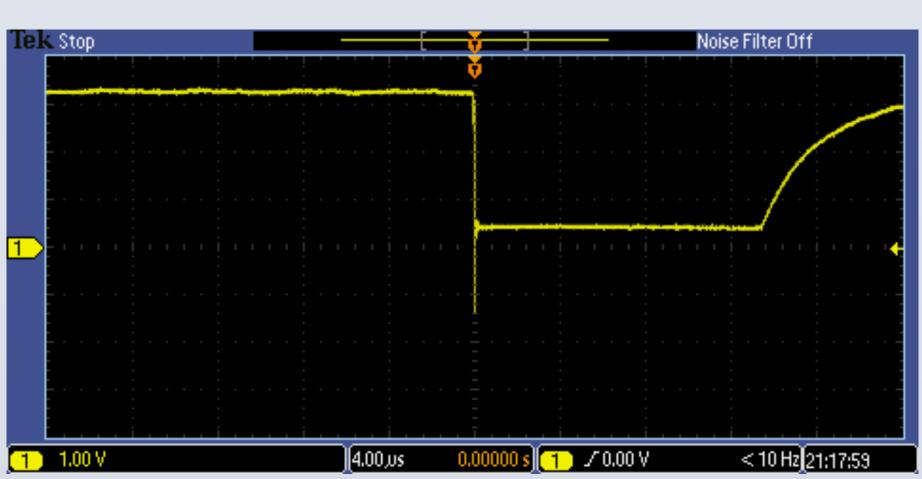
Image 3) This image shows the voltage level that the Raspberry Pi outputs through each of the GPIO pins. The Pi outputs a consistent 3.3V which corresponds to the other two images above.
