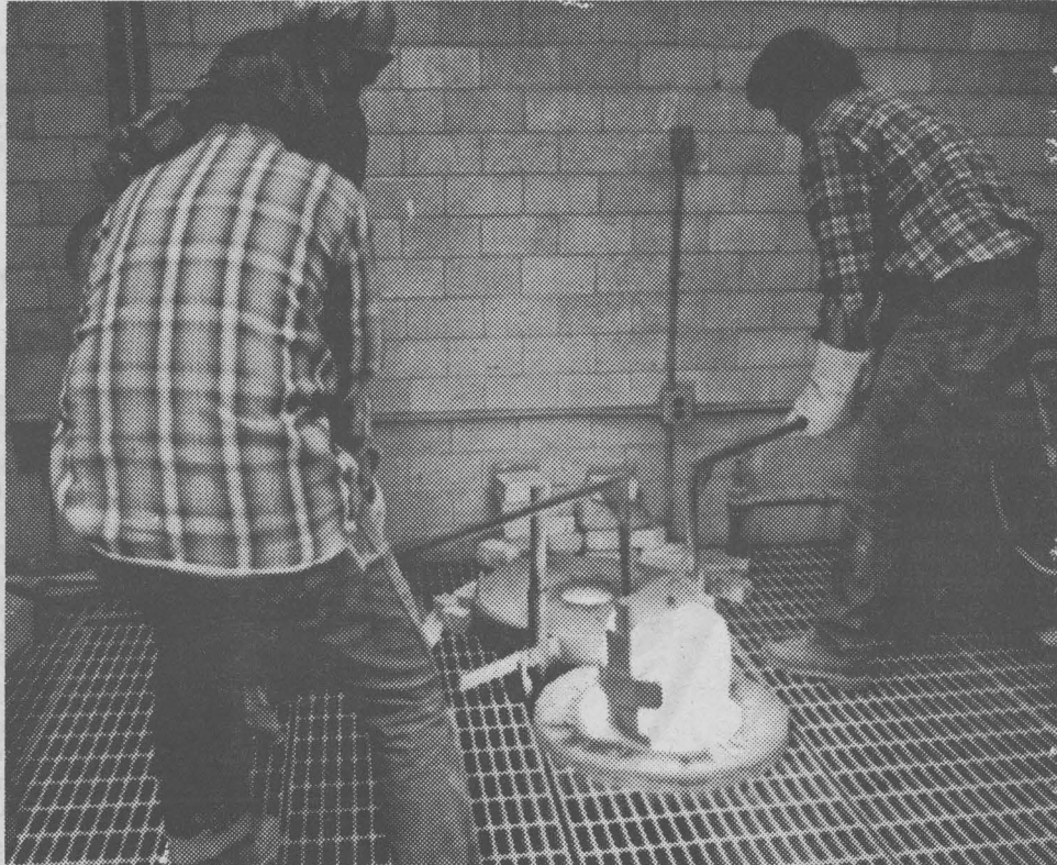
The crucible of molten bronze is lifted from the furnace. Handling this how load are Kevin Radley, Gary Galbraith and Ed Wicklander.
