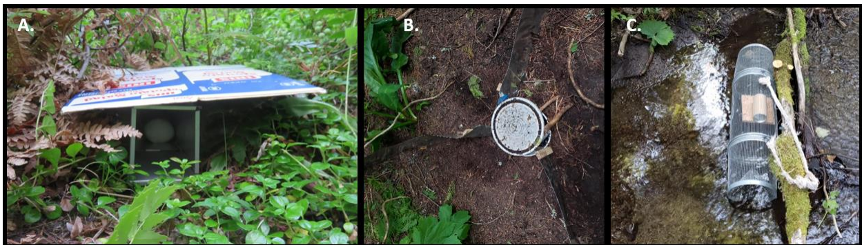
Fig. 2.3. Sherman trap with waxed carton covering to protect from rain (A). Middle bucket from pitfall array showing fencing leading to other buckets (B). Modified funnel trap (C).
