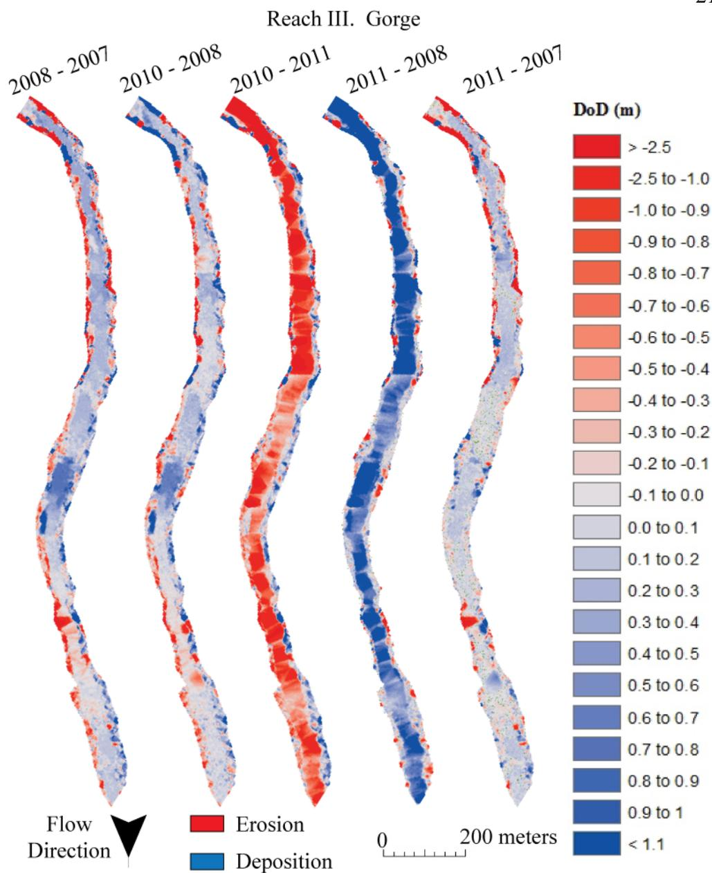
Figure 8: DoD maps of the full channel for a portion of the Gorge Reach showing the deposition and erosion within the Gorge. Some of the apparent change within the channel is due to higher water level in 2007 and 2010; values were resolved in data Table 2.
