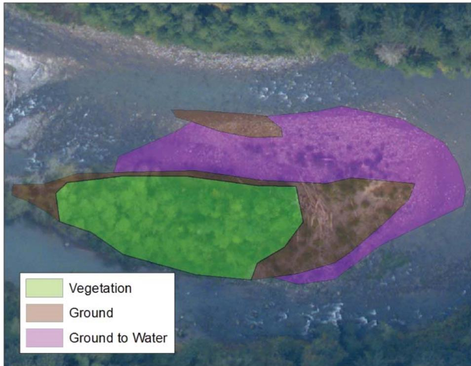
Figure 4: Example of the error model applied to a sediment bar. Each shaded polygon was assigned a specific vertical error uncertainty used for the error propagation model in GCD. Error values were based on project reports provided by Watershed Sciences.
