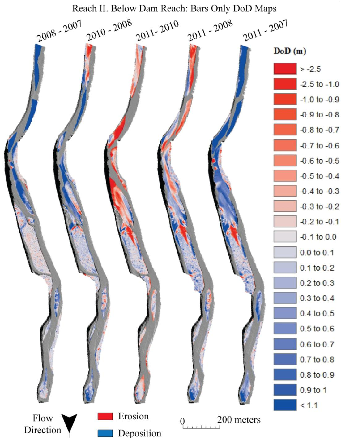
Figure 7: DoD maps for the sediment bars within the 2 km Below Dam Reach. The water surface was removed and the remaining surfaces were differenced to examine how much of the change occurred above the water surface, and to determine how much the water surface influenced the volume estimates.
