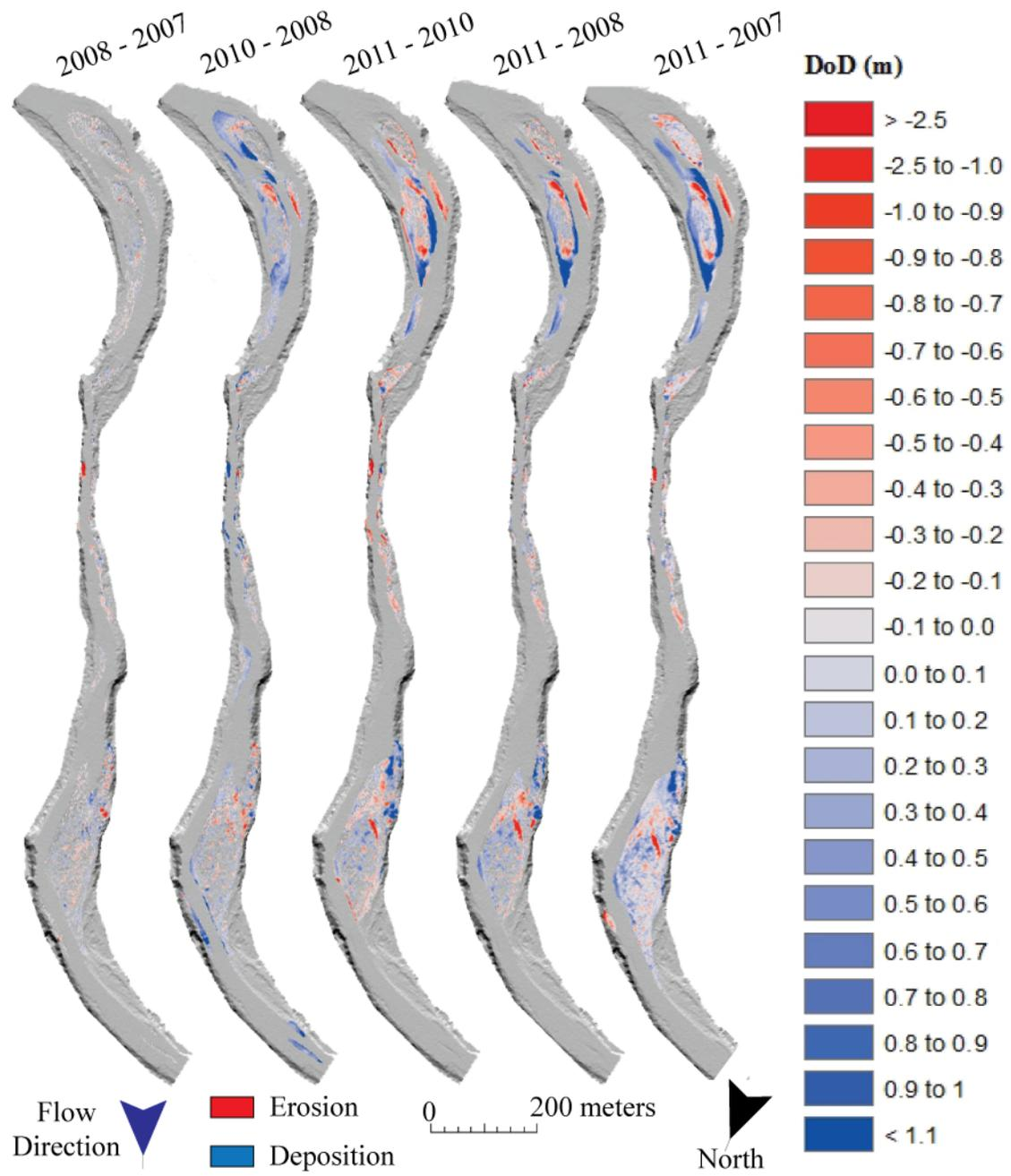
Figure 10: DoD maps for the first 2 km of the Gorge to Bull Run Reach with the water surface removed to more easily show the sediment deposition on the bars immediately downstream from the gorge that is attributed to the sediment pulse from the Marmot Dam removal.
