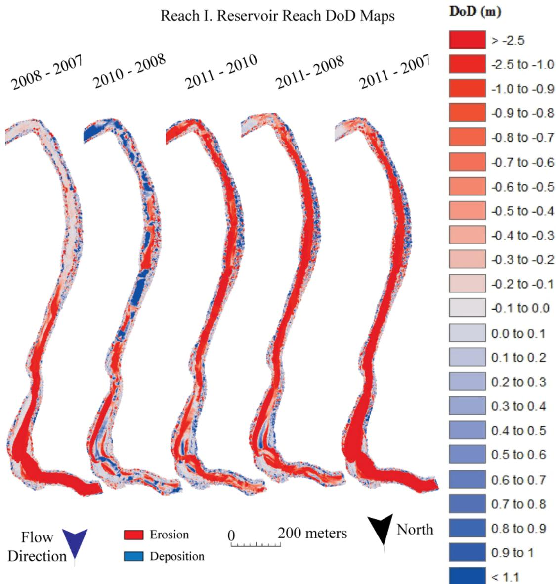
Figure 5: DoD maps for the former reservoir reach located behind the former Marmot Dam showing the change in vertical elevation of the ground surface between LiDAR surveys. Some of the apparent change within the channel is due to higher water levels in 2007 and 2010; values were resolved in data table 2.
