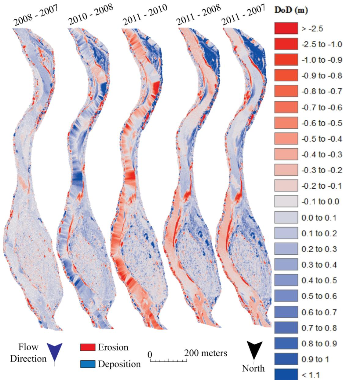
Figure 12: DoD maps for a 2-km section of the Dabney Park to Columbia River reach, the final reach of the Sandy River before it enters the Columbia River. In this reach there was consistent deposition during the study period (2007-2011), but no observed pulse of sediment moving through the reach. Some of the apparent change within the channel is due to higher water levels in 2007 and 2010; values were resolved in Table 2.
