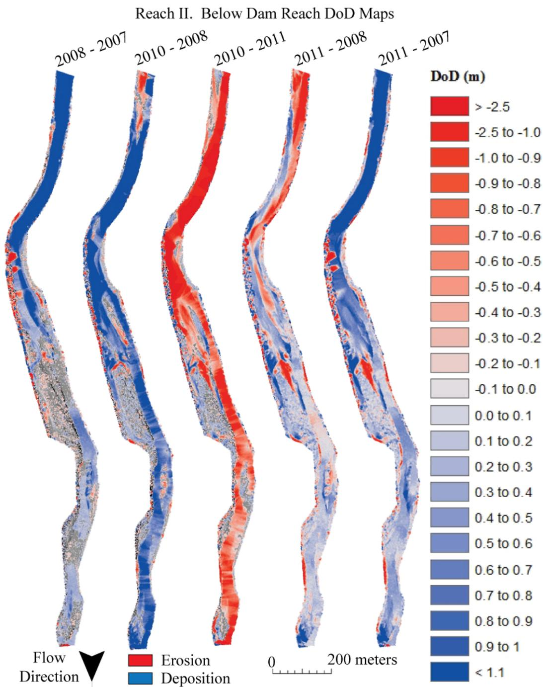
Figure 6: DoD maps for the 2 km Below Dam reach directly below the former Marmot Dam showing the change in vertical elevation of the ground surface between LiDAR surveys. Large volumes of deposition from the dam removal are visible within the reach. Some of the apparent change within the channel is due to higher water levels in 2007 and 2010; values were resolved in Table 2.
