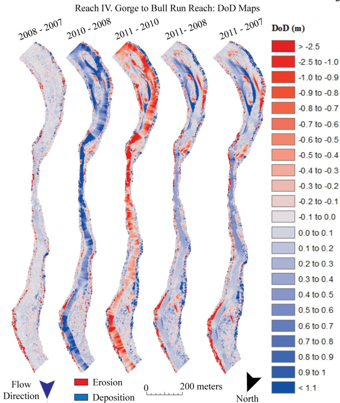
Figure 9: DoD maps of the full channel for the first 2 km of the Gorge to Bull Run Reach showing the deposition on sediment bars near the mouth of the gorge that is evidence for a sediment pulse coming from the former Marmot Dam removal. Some of the apparent change within the channel is due to higher water level in 2007 and 2010; values were resolved in data Table 2.
