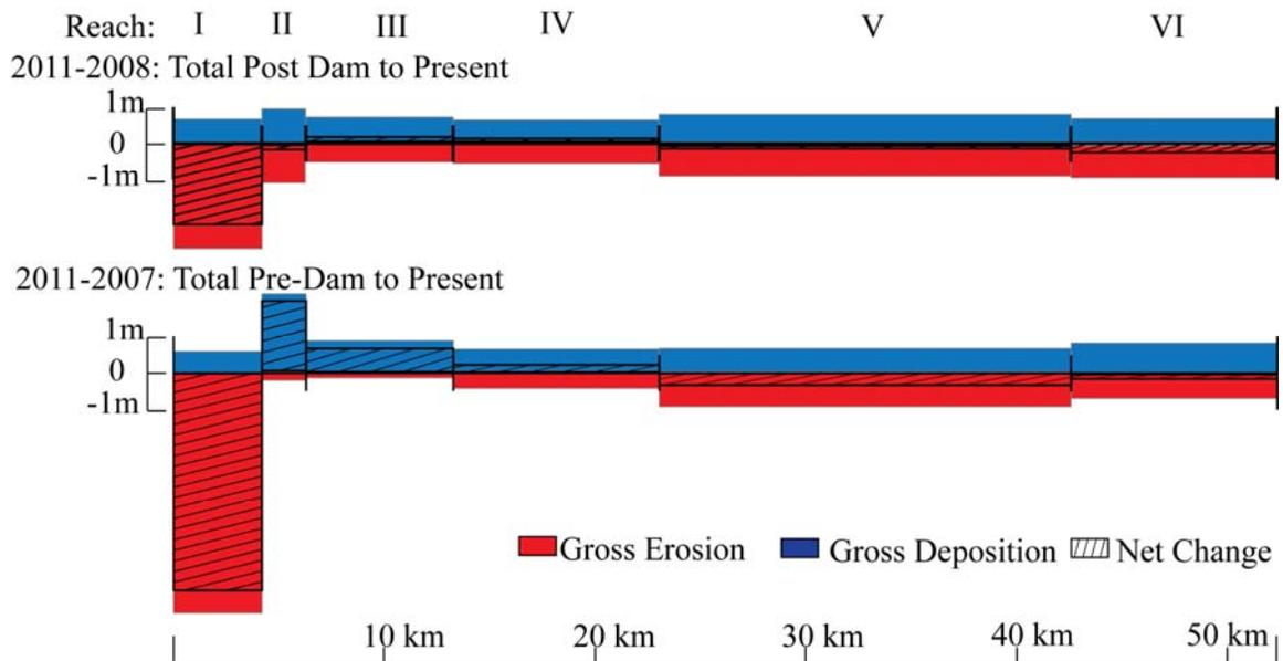
Figure 13: Gross deposition, erosion and net change of each DEM pair during incremental time periods for the Sandy River from the former Marmot Dam Reservoir to the Columbia River. The volumes of sediment from Table 2 (normalized where applicable) were divided by the length and average width of the channel in each reach to show the average vertical change in each section. Reach Labels: I. Reservoir, II. Below Dam, III. Gorge, IV. Gorge to Bull Run, V. Oxbow, VI. Dabney Park to Columbia River.
