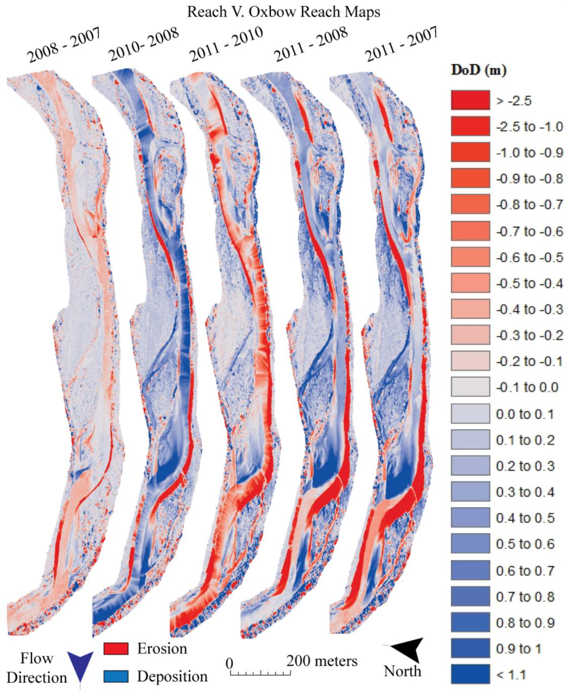
Figure 11: DoD maps for a 2.5 km section of the Oxbow Reach. The DoD depicts erosion and deposition throughout the reach during the study period, with no discernible downstream migration of a pulse of sediment following the Marmot Dam removal. Some of the apparent change within the channel is due to higher water levels in 2007 and 2010; values were resolved in Table 2.
