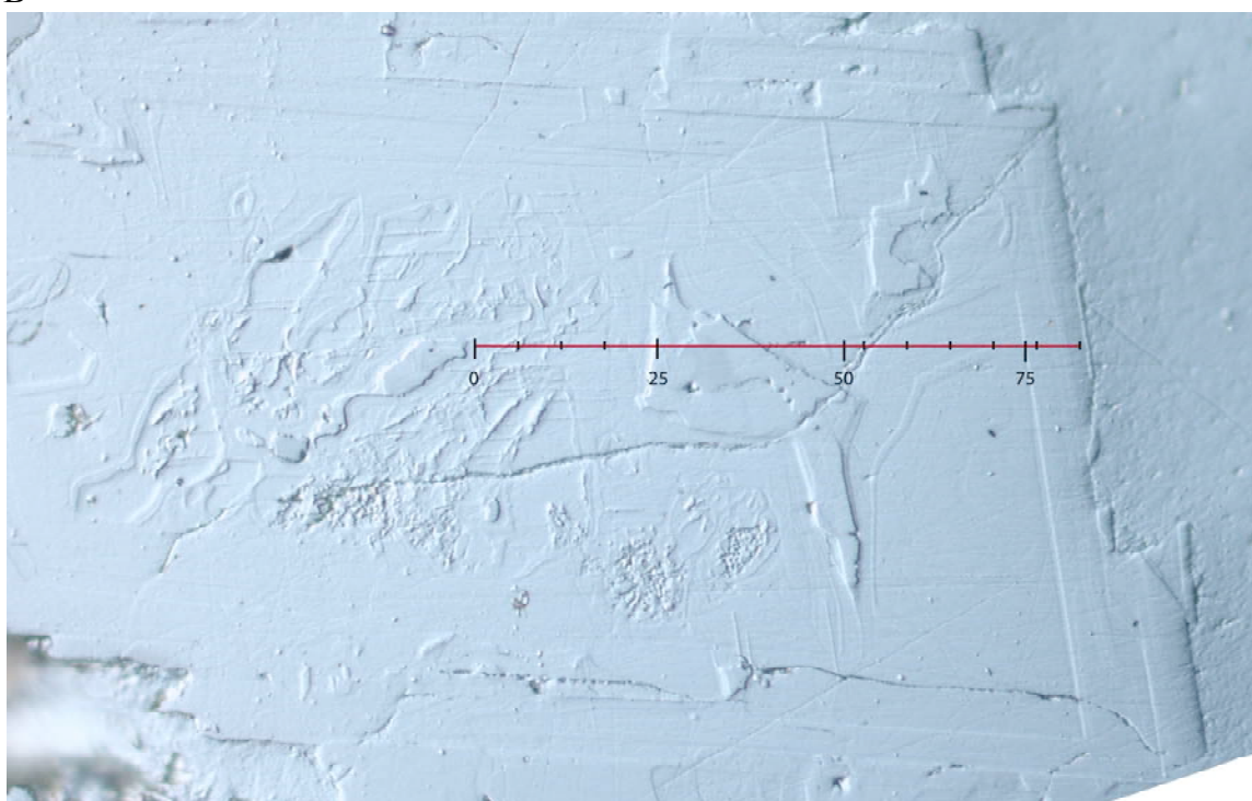
Figure 15. Anorthite content across a traverse for Kwohl Butte (sample 8507092). A) An content (mol %) plotted versus distance from core to rim of sample. B) Nomarski differential interference contrast image of crystal with microprobe traverse plotted for reference. Crystal is classified as IT.
