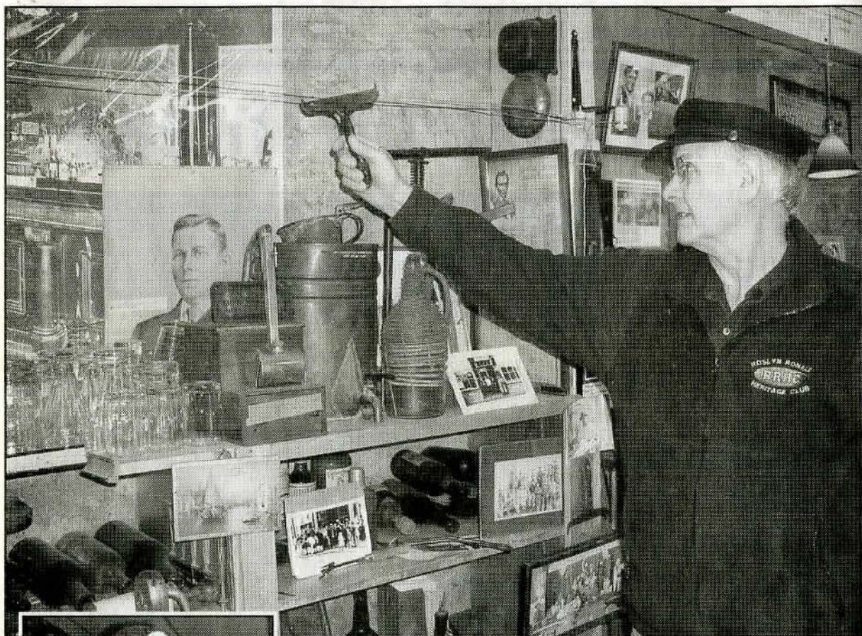
ROSLYN NATIVE Jim Barich demonstrates with a Roslyn Museum display how a Rope Rider signalled for coal cars to be brought back to the surface. While straddling two coal cars, each weighing over a ton, the Rope Rider would hold a metal plate to a charged wire which rang a bell above ground. John Fannin photo
